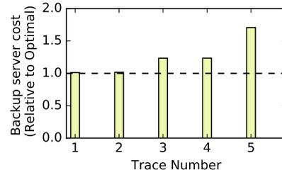
Fig. 11. Cost of backup servers relative to optimal packing for the Eucalyptus cloud traces.
