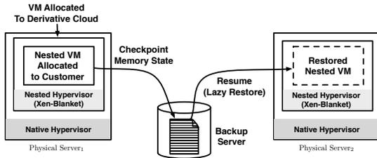
Fig. 3. SpotCheck bounded-time VM migration for moving nested VMs within an IaaS platform.
