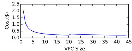
Fig. 15. Cost of running in private cloud mode for different sizes.
