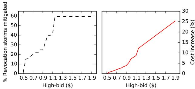
Fig. 14. Two-level bidding reduces impact of revocation storms because only half the servers are affected. As the high-bid is increased, the percentage of storms mitigated increases upto a limit, and so does the cost (compared to single-level bidding).
