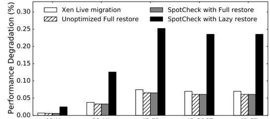
Fig. 13. Performance degradation during migration.
