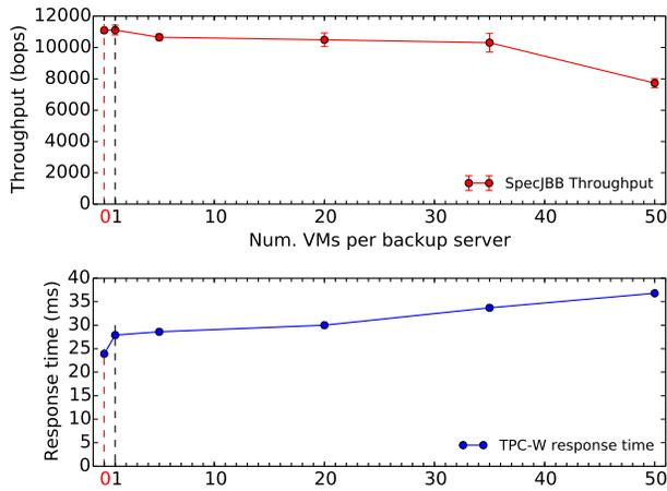
Fig. 7. Effect on performance as the number of nested VMs backing up to a single backup server increases.
