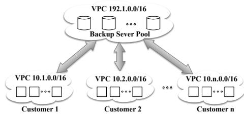
Fig. 4. SpotCheck creates separate VPCs for each customer. Customers can share a pool of backup servers by connecting to backup server VPC. In Amazon EC2, this is done through VPC peering.
