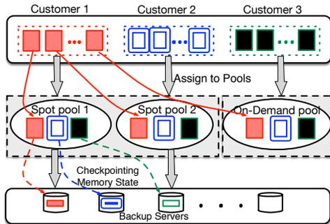
Fig. 5. SpotCheck's architecture using multiple pools.
